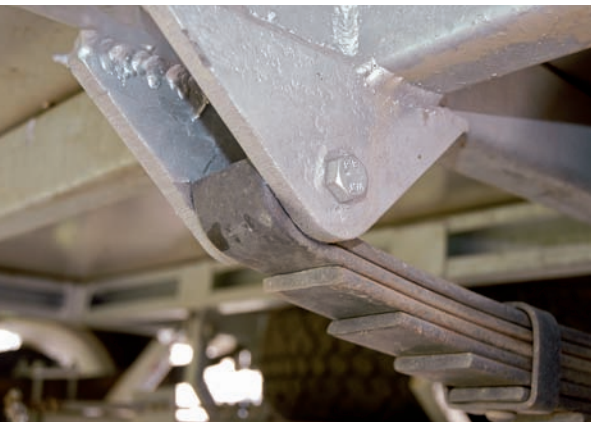
Left Heavy-duty spring mounts bump up off-road confidence. Middle An exterior tap is conveniently placed to the right of the kitchen. Right The Infanta's standard tool kit is a simple but valuable standard feature.
